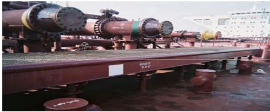
Figure 2.3.5(2)c The safe load of cruciform bollards is stamped permanently on the body
