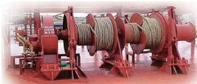
Figure 2.3.5(2)a The safe load of winches is stamped permanently on the body
