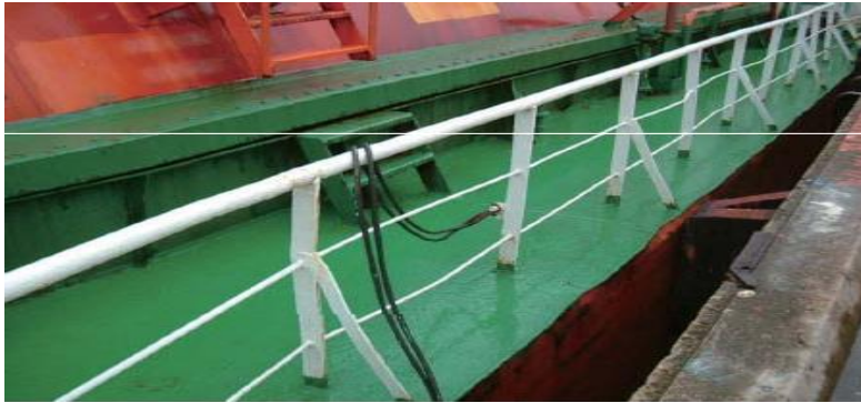
Figure 8.9.3b Bonding installations onboard ships
