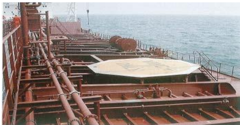
Figure 8.10.5b Arrangement of winching area onboard ships
