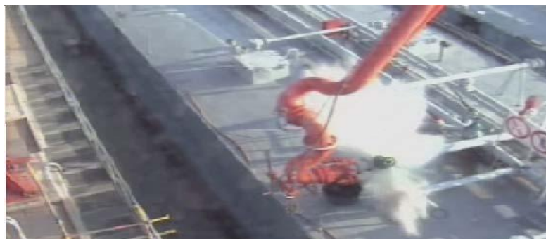
Figure 7.2.5b Falloff accident of cargo arm during cargo operation
