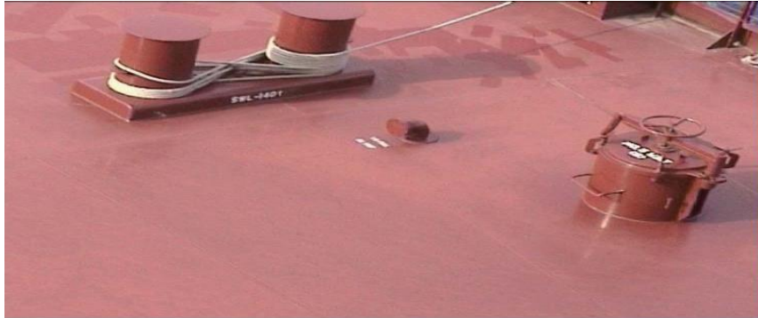
Figure 5.4.5a Sampling and observation arrangements of ballast tank
