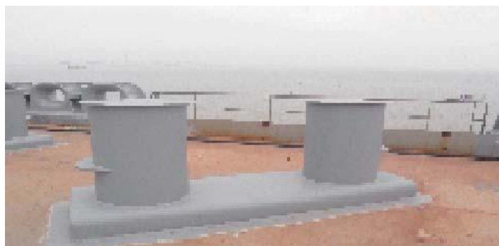
Figure 2.3.5(2)b The safe load of double bollards is stamped permanently on the body
