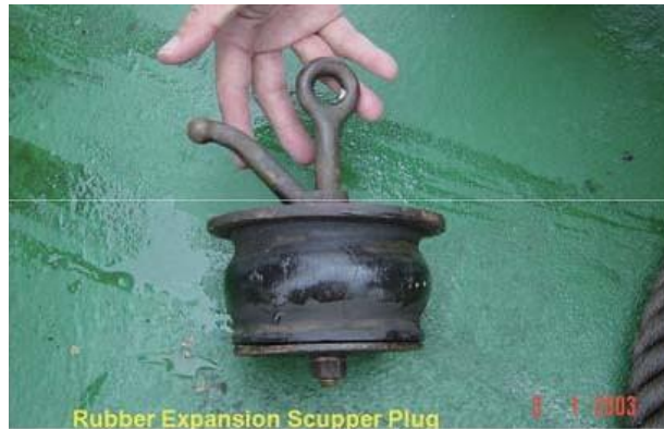
Figure 5.2.5c Closing facility of deck scupper
