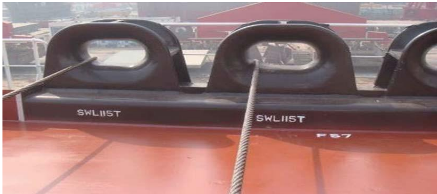
Figure 4.5.7a Closed fairlead marked with SWL
