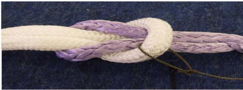
Figure 4.3.14 Synthetic tails connected by cow hitch
