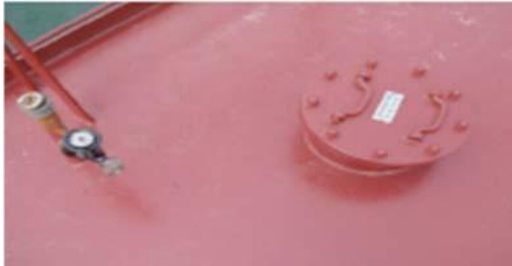
Figure 5.3.4a Sampling and observation arrangements of ballast tank
