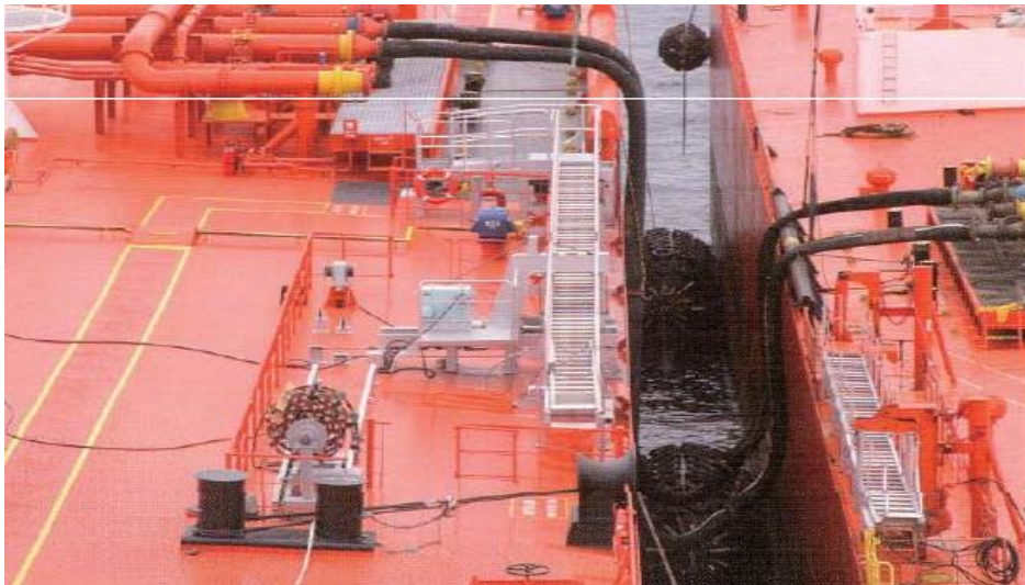
Figure 4.2.4h Ship to ship transfer mooring arrangement
