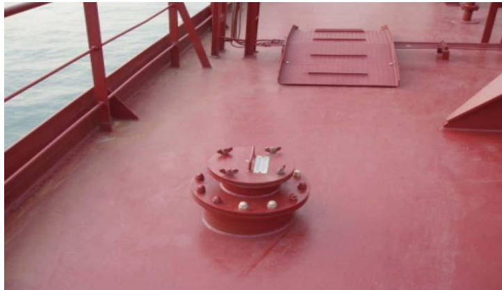
Figure 5.3.4b Sampling and observation arrangements of ballast tank
