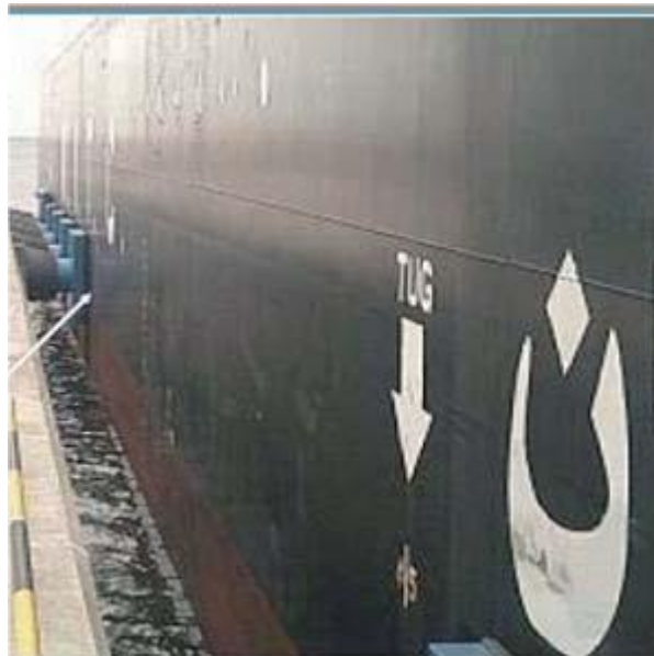
Figure 3.6.2 Marking of tug-pushing location
