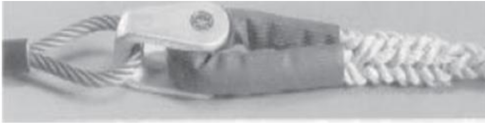
Figure 4.3.13a Synthetic tails connected to a wiring mooring line using Tonsberg shackle
